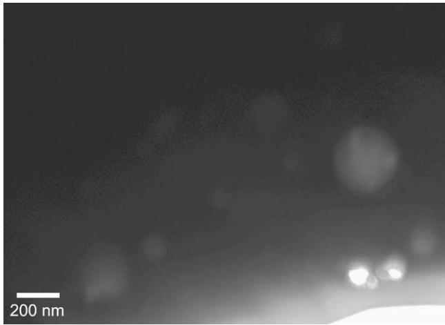
Fig. 5. TEM image showing relatively large fission gas bubbles present in a U-7Mo fuel particle.
